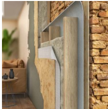
Internal wall insulation
