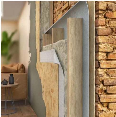
Internal wall insulation
